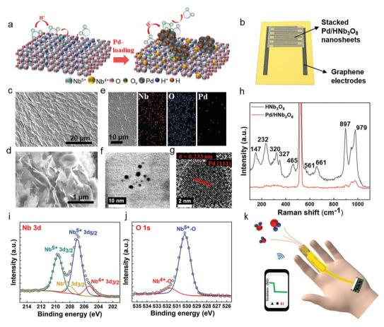
Fig. 1 Schematics of (a)  $HNb_3O_8$  and H-atom-enriched Pd-doped  $HNb_3O_8$  and (b) the  $Pd/HNb_3O_8$  humidity sensor. (c and d) Surface morphology and (e) SEM-EDX images for the Nb, O, and Pd distributions of the  $Pd/HNb_3O_8$  nanosheets. (f) TEM image of Pd nanoparticles on ultrathin  $HNb_3O_8$  nanosheets. (g) HRTEM analysis of the Pd nanoparticles. (h) Raman spectrum of pristine  $HNb_3O_8$  and  $Pd/HNb_3O_8$ . XPS spectra of (i) Nb 3d and (j) Nb 3d
