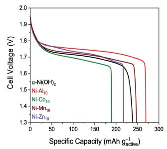
Fig. 5 Voltage vs. specific capacity for 5th cycle discharge of Ni-Zn sponge cells for powder-composite cathodes containing unsubstituted  $\alpha$ -Ni(OH)<sub>2</sub>, aluminum-substituted (Ni-Al $_{10}$ ), cobalt-substituted (Ni-Co $_{10}$ ), manganesesubstituted (Ni-Mn<sub>10</sub>), or zinc-substituted (Ni-Zn<sub>10</sub>) nanosheets at a massnormalized current of 84.4 mA  $g_{active}^{-1}$  between 1.3–2.0 V.
