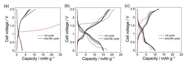
Fig. 4 Charge-discharge performance of symmetric NiNc-NiNc batteries assembled with distinct electrolytes: (a) EC/DMC, (b)  $[C_2C_1im][FSA]$ , and (c) 50 mol% Na[FSA]-[C<sub>2</sub>C<sub>1</sub>im][FSA]. Current density and cut-off voltages were set as 50 mA  $g^{-1}$  and 0–2.5 V.
