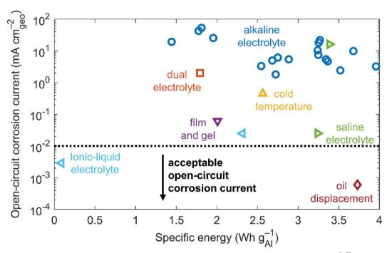
Fig. 2 Open-circuit corrosion currents *versus* respective specific energies for reported corrosion-mitigation strategies.  $^{9-32}$  We group anode alloying, electrolyte additives, anode grain sizes, and anode crystal orientations into one category characterized by the use of alkaline electrolyte. Methods yielding open-circuit corrosion currents below 0.01 mA cm<sub>geo</sub> $^{-2}$  are acceptable. See also Table S1 (ESI†).
