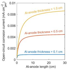
**Fig. 1** Open-circuit corrosion current *versus* Al-anode length and thickness while requiring a self-discharge rate of  $2\% \text{ y}^{-1}$ . We calculate open-circuit corrosion current using the equation in Table 2.
