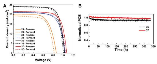
Fig. 11 (A) Reverse J-V curves of the champion PSCs of composition No. 29, 30, 36, and 37 using 1.0 M perovskite precursor solutions with 5% excess  $Pb^{2+}$ . (B) Continuous MPP tracking results under 1 Sun irradiation in a  $N_2$  atmosphere for devices of composition No. 36 and 37.
