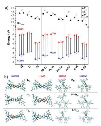
Fig. 3 (a) DFT-calculated (PBE0/6-31G\*\* level) HOMO-LUMO gaps (a) and frontier molecular orbital energies (b) for the  $T_2$  (solid circles),  $T_3$  (open circles) and T<sub>2,3</sub> (solid triangle) models. (b) HOMO and LUMO topologies of the directly connected  $T_2$  dimeric models and  $Tr_{2.3}$  trimeric models chosen as representatives (see Fig. S6 (ESI†) for the remaining compounds)
