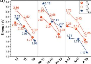
Fig. 7 (a) Calculated band-gaps and bandwidths for the conduction bands (CBs) and valence bands (VBs) of all the hexa-substituted truxenebased 2D COFs. (b) Comparison of the calculated band-gaps for all the 2D polymers under study. The zero energy is taken to correspond to the valence band maximum.
