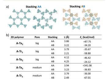
**Fig. 9** (a) Pictorial top views of the two different stacking AA and AB configurations. (b) Computed data of the fully optimized inter-layer stacking distance (in Å) and inter-layer cohesive energy (in kcal mol<sup>-1</sup>), defined as the difference between the total energy crystal-bulk (with one layer per unit cell) and the isolated single-layer, for the **A-T<sub>2</sub>** and **A-T<sub>3</sub>** compounds.
