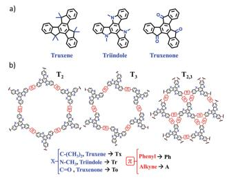
Fig. 1 General chemical structures of the conjugated cores (a) and 2D polymers (b) examined in this study with the notation used throughout the text. Note that  $T_2$  and  $T_3$  polymers refer to tri-substituted materials with different linkage positions (2,7,12 in  $T_2$  and 3,8,13 in  $T_3$ ), while  $T_{2,3}$ corresponds to hexa-substituted materials in the 2,3,7,8,12 and 13 positions
