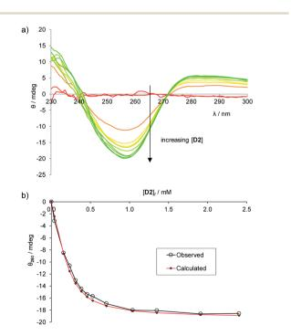
Fig. 3 (a) CD spectra from the titration of p-glucose into 1 (0.25 mM) in aqueous phosphate buffer (10 mM, pH = 7.4). Cell path length = 0.1 cm, 16 scans accumulated at each concentration. (b) Curve-fitting analysis of the CD signal at 260 nm, assuming a 1 : 1 binding model.  $K_a = 17\ 200\ M^{-1}$ .
