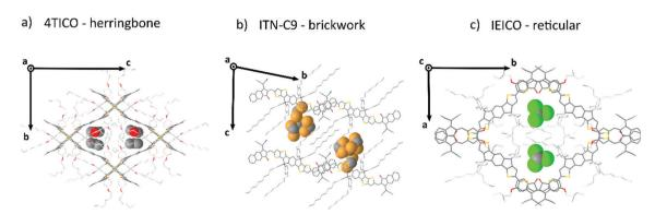
Fig. 6 Graphic representation of the three most common molecular packing for A-D-A molecules. A section of the unit cell of 4TICO (a), ITN-C9 (b) and IEICO (c) is shown with their respective solvent inclusions:  $C_3H_6O$ ,  $CH_2Br_2$  and  $CHCl_3$ , which have been highlighted using a space fill model.
