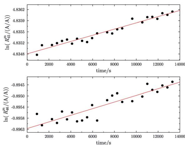
Fig. 8 Logarithms of  $R_{45}^{\text{m}}$  (top) and  $R_{46}^{\text{m}}$  (bottom) against time during the measurement of parent gas B ( $^{13}\text{C}$  enriched material). The gas was heated prior to the measurement for 13 h using a Bunsen burner ( $\vartheta \approx 1800^\circ\text{C}$ ).
