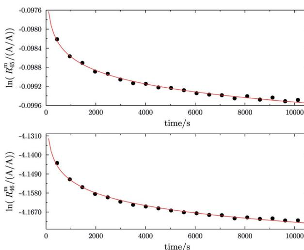
Fig. 1 Plot of  $\ln(R_{45}^m)$  against time (top) and  $\ln(R_{46}^m)$  against time (bottom) in case of blend b1. The black dots are the measured ratios, the red lines are fits using the generic equation  $\ln(R_X^m) = a_1 \times \ln(t) + a_0$ . Both graphs show that the  $\ln$  of both ratios does not linearly increase over time.
