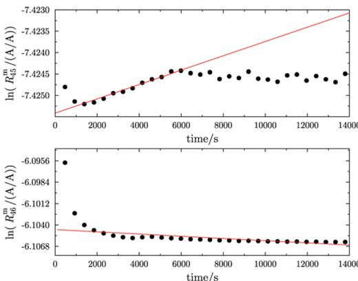
(c) Logarithms of  $R_{45}^m$  and  $R_{46}^m$  against time during the measurement of parent material A. Prior to the measurement, an aliquot of the gas was filled in one of the gas spheres. Previous to the filling with gas A, a platinum band was placed into the sphere. Subsequently, the sphere was heated for 39.5 h with a Bunsen burner ( $\vartheta \approx 1800$  °C).
