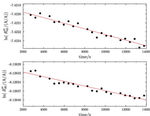
(b) Logarithms of  $R_{45}^m$  and  $R_{46}^m$  against time during the measurement of parent material A. Prior to the measurement, an aliquot of the gas was filled in one of the gas spheres and heated for 48 h with a Bunsen burner ( $\vartheta \approx 1800$  °C). (Six outliers were removed.)
