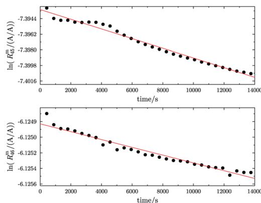
(a) Logarithms of  $R_{45}^m$  (top) and  $R_{46}^m$  (bottom) against time during the measurement of parent material A ( $^{12}\text{C}$  enriched material). The gas was heated prior to the measurement for 25 h with a Bunsen burner ( $\vartheta \approx 1800$  °C).
