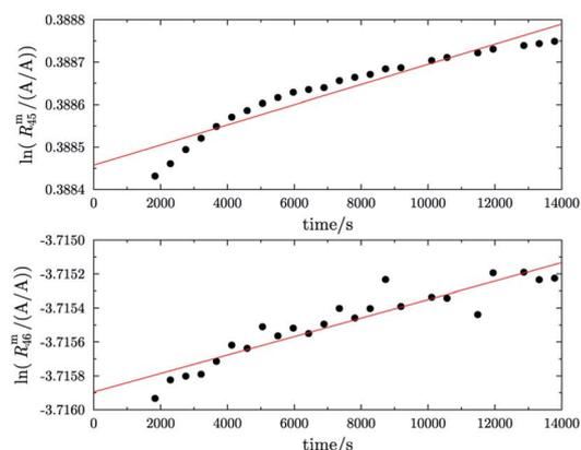
(c)  $\ln(R_{45}^m)$  against time (top) and  $\ln(R_{46}^m)$  against time of blend b2 (bottom). The blend was heated with a Bunsen burner for 19.5 h before the measurement. The red line in both graphs indicates a linear fit.
