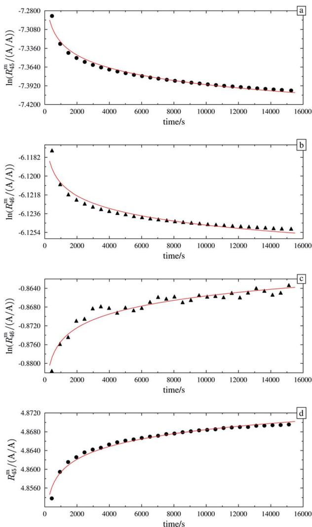
Fig. 7  $\ln(R_{45}^{\text{m}})$  against time and  $\ln(R_{46}^{\text{m}})$  against time of the  $^{12}\text{C}$  enriched material A (graphs (a) and (b)).  $\ln(R_{45}^{\text{m}})$  and  $\ln(R_{46}^{\text{m}})$  against time of the  $^{13}\text{C}$  enriched material B (graphs (c) and (d)). The red lines in all four plots are fitted logarithmic curves.
