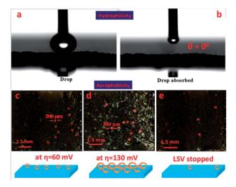
Fig. 6 Wettability test of the Cuf@Ni<sub>5</sub>P<sub>4</sub> surface: (a) before; and (b) after placing a liquid drop with a contact angle of 0°. (c-e) Optical images with a schematic diagram in the bottom panel showing the bubble formation behavior on the Cuf@Ni<sub>5</sub>P<sub>4</sub> surface at different overpotentials and at the end of LSV.
