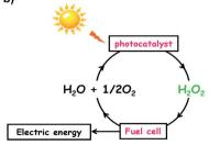
Scheme 1 (a) Solar hydrogen cycle and (b) solar oxygen cycle.
