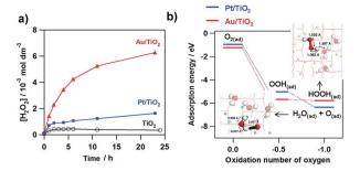
Fig. 4 Time courses for the M(Au and Pt)/TiO<sub>2</sub>-photocatalyzed ORR to  $H_2O_2$  under UV-light irradiation ( $\lambda > 300$  nm, light intensity  $I_{290-390~\rm nm} = 3~\rm mW~cm^{-2}$ ) and unmodified TiO<sub>2</sub> system for comparison. (b) Adsorption energy change with the  $M_{28}/\rm TiO_2$ -photocatalyzed two-electron ORR (M = Au and Pt. Figure (b) is taken from ref. 54.
