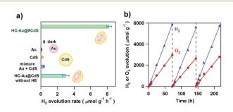
Fig. 5 (a) The comparison of the  $H_2$  evolution rate for HC-Au( $d_{Au}=5.5$  nm)@#CdS(ICdS = 1.9 nm), Au colloid, CdS, and a mixture of Au and CdS under red-light illumination ( $\lambda_{ex}=640$  nm) or dark conditions. (b) Repeated water splitting by HC-Au( $d_{Au}=12.1$  nm) @#CdS(ICdS = 2.1 nm) under red-light illumination. Figures are taken from ref. 59.
