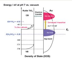
Scheme 2 Energy diagram of the Au/TiO<sub>2</sub> plasmonic electrode with the density of states of TiO<sub>2</sub> and energy distribution of the hot carriers in Au NPs with the intraband transition *via* the surface plasmon decay.
