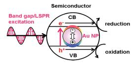
Fig. 2 Local electromagnetic field-enhanced mechanism.
