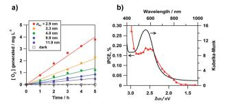
Fig. 3 (a) Time courses for the rate of  $O_2$  generation. (b) IPCE action spectrum for the photoelectrochemical WOR of the Au/TiO<sub>2</sub>/FTO photoelectrodes with the absorption spectrum for comparison. Figure (a) is taken from ref. 41.
