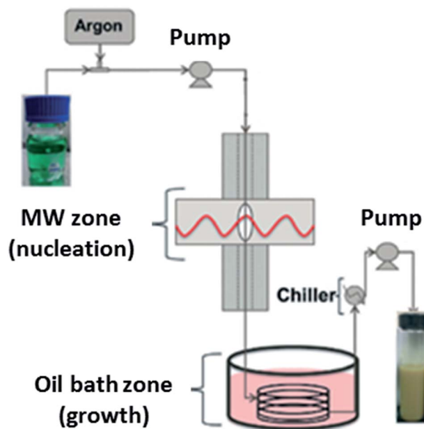
Fig. 7 Schematic diagram of the gas liquid segmented continuous flow reactor for synthesis of MOF-74(Ni) developed by Albuquerque et al. 166 Reproduced from ref. 166 with permission from the Royal Society of Chemistry.
