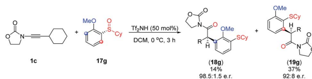
Scheme 5 Asymmetric rearrangement with chiral enantiopure sulfoxides.
