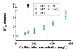
Fig. 2 Photodegradation half-lives of clothianidin (DT $_{50}$ , hours) for the series of nanoformulations (NFA, NFB and NFC), the commercial formulation (Com) and pure clothianidin (Al). Tests were carried out across a wide range of concentrations either in water (coloured symbols) or in fertiliser background (black symbols). The dashed line indicates the water solubility of clothianidin (340 mg L $^{-1}$  (ref. 7)).
