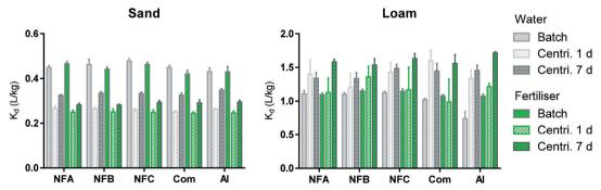
Fig. 3 Sorption coefficients (K<sub>d</sub>, L kg<sup>-1</sup>) measured by batch method (plain) and centrifugation method after 1 (diagonal strips) or 7 days (horizontal strips). Data obtained in water are in grey and with fertiliser, in green. Error bars represent standard deviation for triplicates (all values are available
