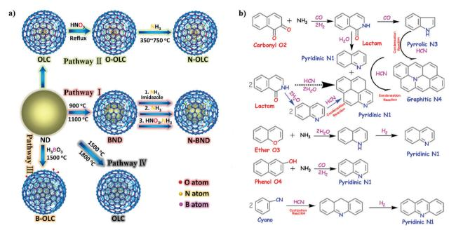
Fig. 8 (a) Sketch for the production of UNDDs and related materials. (b) The possible evolution pathways of different nitrogen species during the preparation process of nitrogen-modified UNDDs (two hexatomic rings as ideal starting model structures in different pathways). Reproduced from ref. 156 with permission from American Chemical Society, copyright 2014.
