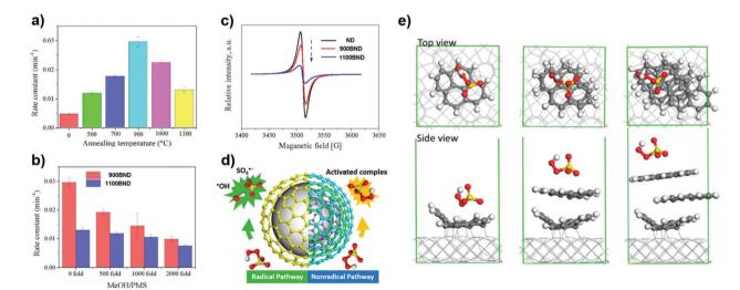
Fig. 12 (a) Influence of different annealing temperatures on phenol removal. (b) Quenching effect of phenol removal on BNDs with different graphitic degrees. (c) ESR spectra of UNDDs. (d) Illustrations of radical and non-radical oxidations on UNDDs. (e) Theoretical modulation of BNDs with different graphitic layers, reprinted from ref. 170 with permission from Elsevier, copyright 2018
