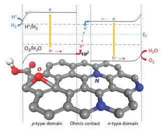
Fig. 27 Mechanism<sup>242</sup> suggested for the photocatalytic water splitting on nitrogen-doped graphene. Reproduced from ref. 70 with permission from Elsevier, copyright 2017.
