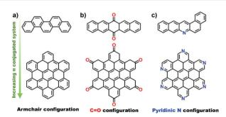
Fig. 29 Polycyclic aromatic hydrocarbon (PAH) organic molecules with single (a) armchair, (b) C=O and (c) pyridinic N configurations as model catalysts.
