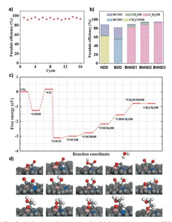
Fig. 18 (a) Faradaic efficiencies for  $\rm CH_3CH_2OH$  in 16 consecutive CRR runs on BNND3 at 1.0 V. (b) Faradaic efficiencies for the CRR on different catalysts at 1.0 V. (c) Free energy diagrams for the CRR on BBNDs. (d) Energetically favorable structures for elementary steps of the CRR on BBNDs. Gray dots, pink dots, blue dots, red dots and white dots represent C, B, N, O and H atoms, respectively, reprinted from ref. 207 with permission from Wiley, copyright 2017.
