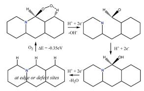
Fig. 23 The ORR mechanism suggested for N-doped graphene edges, evidencing how O2 adsorbs at carbon adjacent to a N-atom. Based on indications of ref. 231 with permission from Royal Society of Chemistry, copyright 2016.
