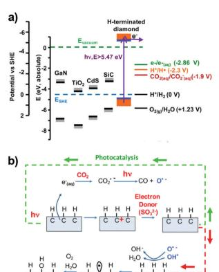
Fig. 20 (a) Energy band diagram of H-terminated diamonds and some other semiconductors, together with some related redox reactions. (b) Schematic illustration of relevant chemical and photochemical processes, reprinted from ref. 216 with permission from Elsevier, copyright 2017
