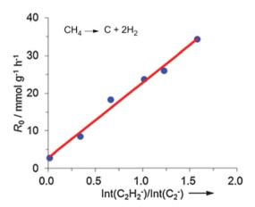
Fig. 21 Initial rate of reaction in CH<sub>4</sub> decomposition at 850 °C versus the  $C_2H_2^-/C_2^-$  ratio in SIMS spectra of ND samples, which were annealed in the 900-2000 °C temperature range. Adapted from ref. 131 with permission from Royal Society of Chemistry, copyright 2014.
