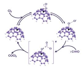
Fig. 26 Catalytic mechanism of CO chlorination on a fullerene hemisphere with controlled curvature, as a model for OLC-like carbon nanospheres. Reproduced from ref. 240 with permission from Wiley, copyright 2015.
