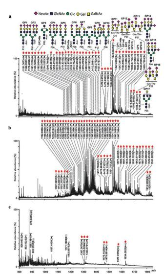
Fig. 3 The performance of polySD-SiO $_2$  (a and b) and commercial ZIC-HILIC (c) toward glycopeptides using tryptic digests of bovine fetuin and bovine serum albumin (BSA) at molar ratios of 1:100 (a and c) and 1:3000 (b). Glycopeptides are labelled with their corresponding glycans or red asterisks.
