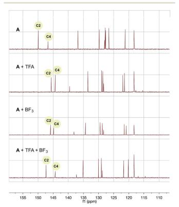
Fig. 3  $^{13}$ C NMR of A with trifluoroacetic acid and/or BF<sub>3</sub> additive in CD<sub>3</sub>CN/H<sub>2</sub>O (1 : 1). CD<sub>3</sub>CN solvent peak was used as a reference.
