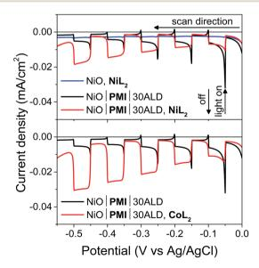
Fig. 4 Linear sweep voltammetry measurements with 10 s light on/off cycles on a NiO working electrode with 0.5 mM NiL<sub>2</sub> (blue) and on a single NiO|PMI|30ALD working electrode without catalyst (black) and with 0.5 mM NiL<sub>2</sub> or 0.5 mM CoL<sub>2</sub> (red) (conditions: 0.1 M H<sub>2</sub>SO<sub>4</sub> and  $0.1 \text{ M Na}_2\text{SO}_4 \text{ in } 1:1 \text{ H}_2\text{O}: \text{MeCN}, 5 \text{ mV s}^{-1}$ ).
