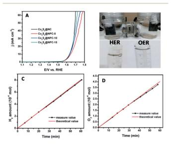
Fig. 5 (A) OER polarization curves for  $\text{Co}_9\text{S}_8$ @NPC-5,  $\text{Co}_9\text{S}_8$ @NPC-10,  $\text{Co}_9\text{S}_8$ @NPC-15 and  $\text{Co}_9\text{S}_8$ @NC electrodes at 10 mV s<sup>-1</sup> in 1.0 M KOH. (B) A photograph of overall water splitting and the gas collection equipment. (C and D) The dependence of the theoretically calculated and experimentally measured hydrogen and oxygen amounts on time during electrocatalytic water splitting using  $\text{Co}_3\text{S}_8$ @NPC-10.
