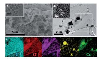
Fig. 1 (A) and (B) SEM and TEM images of  $Co_9S_8$ @NPC-10. The insets in (A) and (B) are the corresponding high magnification SEM and high resolution TEM images. (C) Corresponding elemental mapping analysis of the selected area from (B).
