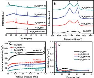
Fig. 2 (A) XRD patterns, (B) Raman spectra, (C)  $N_2$  adsorption—desorption isotherms and (D) pore size distribution curves of  $Co_9$ - $S_8$ @NPC-5,  $Co_9S_8$ @NPC-10,  $Co_9S_8$ @NPC-15 and  $Co_9S_8$ @NC.
