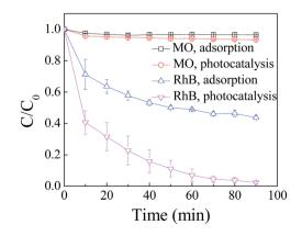
Fig. 1 Degradation of RhB and MO by adsorption and photocatalysis. The concentration of RhB and MO was 15 mg  $\rm L^{-1}$  and the dosage of  $\rm Znln_2S_4$  was 0.1 g  $\rm L^{-1}$ .
