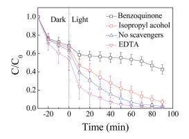
Fig. 4 Photocatalytic degradation of RhB by  $ZnIn_2S_4$  under visible light irradiation in the presence of scavengers: EDTA, benzoquinone, and isopropyl alcohol were used to capture holes,  ${}^{\bullet}O_2{}^{-}$ , and  ${}^{\bullet}OH$ , respectively.
