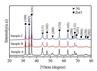
$\label{eq:fig.1} \textbf{Fig. 1} \quad \textbf{XRD patterns of the Ni/ZnO composites prepared with different solvent solutions}.$
