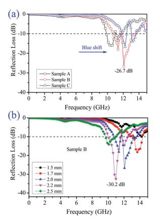
Fig. 9 (a) Reflection loss (RL) of the different Ni/ZnO composites with a thickness of 2.0 mm and (b) RL of the core-shell Ni@ZnO (Sample B) composite with various thicknesses.
