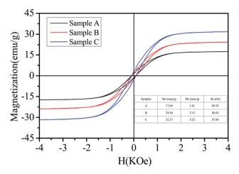
Fig. 6 Magnetization curves of the various Ni/ZnO composites measured at room temperature (the inset is the summarized table of the magnetic properties of Ni/ZnO).
