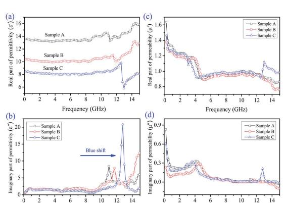
Fig. 7 Frequency-dependence on the (a) real and (b) imaginary parts of the complex permittivity ( $\varepsilon_r = \varepsilon' - j\varepsilon''$ ); (c) real and (d) imaginary parts of the complex permeability ( $\mu_r = \mu' - j\mu''$ ) of Ni/ZnO paraffin composite samples.
