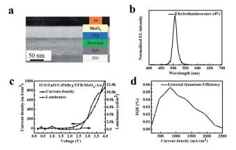
Fig. 7 (a) Device structure of the CsPbBr $_3$  perovskite LEDs. Schematic and the cross-sectional TEM image of the device: ITO/ZnO/perovskite/TFB/MoO $_x$ /Au. (b) Normalized EL spectrum of the CsPbBr $_3$  perovskite thin film-based LEDs at the applied voltage of 4 V. (c) Current density and luminance for the CsPbBr $_3$  perovskite LED measured at room temperature. (d) The external quantum efficiency (EQE) versus current density curves of this LED.
