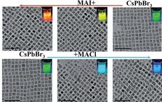
Fig. 4 TEM images of the CsPbBr $_3$  NCs after treatment with various quantities of MAI (up) and MACI (down). The insets show the evolution of emission colors (under a UV lamp,  $\lambda_{\rm ex}=365$  nm) from crude CsPbBr $_3$  NCs to composited perovskite NCs. Scale bars correspond to 50 nm.
