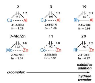
Fig. 17 Comparison of key distances (Å) and angles (°) from X-ray ( $TM \cdots M$ ) structures of coordinated Al-H and Zn-H bonds. Trends confirmed by DFT studies.
