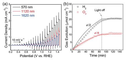
Fig. 4 (a) Current–potential curves obtained from  $Ta_3N_5$  photoanodes with different film thicknesses under simulated AM 1.5G light, and (b) time course of  $O_2$  (open circles) and  $H_2$  (open squares) gas evolution from a  $Ta_3N_5$ (570 nm)/Ta/Ti photoanode held at 1.23 V vs. RHE and a Pt counter electrode, respectively, under simulated AM 1.5G light. Solid curves represent the total charges estimated from the photocurrent.
