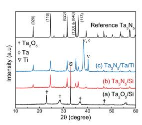
Fig. 2 XRD patterns for (a)  $Ta_2O_5/Si$  and (b)  $Ta_3N_5/Si$  obtained from the nitridation of  $Ta_2O_5/Si$ , and (c)  $Ta_3N_5/Ta/Ti$  after the transfer process. The standard pattern for the  $Ta_3N_5$  phase (PDF# 89-5200) is displayed at the top as a reference.
