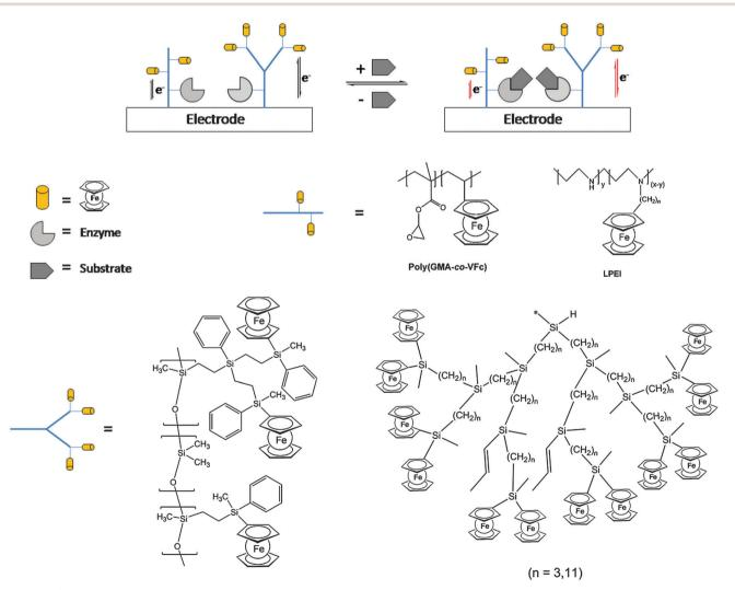
Scheme 13 Sketch of the enzyme activity influencing the redox interaction of the redox polymer with the electrode surface for selected polymer architectures.
