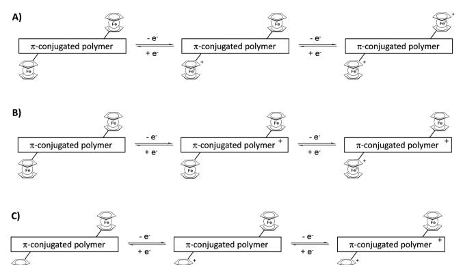
Scheme 17 Sketch of combinations of redox steps in the main chain and/or at the pendant units enabling multicolored electrochromism
