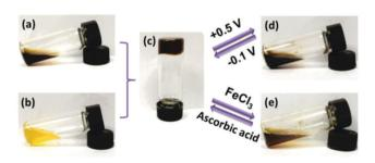
**Fig. 2** Redox switchable sol-gel system. Reproduced from ref. 35 with permission from The Royal Society of Chemistry.
