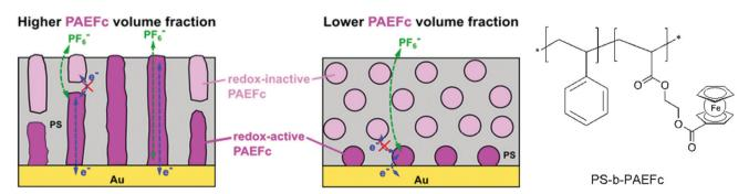
Scheme 16 Microdomains of different sizes and shapes in thin films of ferrocene-containing diblock copolymers (left, reprinted with permission from ref. 11. Copyright (2015) American Chemical Society) and sketch of the polymer structure (right).
