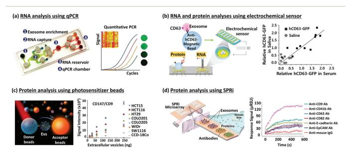
Fig. 2 Devices for EV isolation and analysis. (a) RNA analysis using qPCR.<sup>58</sup> (b) RNA and protein analysis using an electrochemical sensor.<sup>59</sup> (c) Protein analysis using photosensitizer beads.<sup>60</sup> (d) Protein analysis using SPRi.<sup>42</sup> Reproduced from ref. 42 and 58-60 with permission from the Nature Publishing Group, Elsevier, and American Chemical Society.
