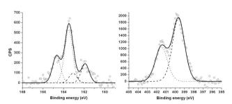
Fig. 6 High-resolution S 2p<sub>3/2</sub> (left) and N 1s (right) XPS data from SAMs of L<sup>3</sup>, produced from methanol solution. Empty circles represent experimental data, dashed and dotted lines correspond to bound and unbound thiols, respectively, in S 2p region (left) and two distinct environments of nitrogen atoms in N 1s spectrum (right). Solid lines show envelopes of the fitted peaks.
