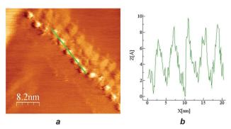
(a) STM image of a representative chain of beads from [Fe(bpp)<sub>2</sub>][BF<sub>4</sub>]<sub>2</sub> drop cast onto HOPG, with widths of 2.5 nm and heights of 7 Å. (b) Profile over the five beads highlighted in (a).
