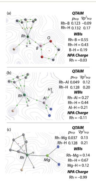
Fig. 3 Electron density contour plots with over-layered calculated structures from QTAIM of (a)  $[Cp*Rh(H)_2(Bpin)(SiEt_3)]$  presented in the  $\{RhBO\}$  plane, (b) 1 presented in the  $\{RhAlH1\}$  plane and (c) 3 presented in the  $\{RhMgN\}$  plane. For X–H bonds (X = Rh, B, Al, Mg) data are given as the mean, green dots are bond critical points, red dots ring critical points.
