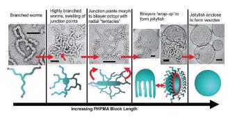
Fig. 7 Preparation of non-spherical micelles by RAFT-mediated aqueous dispersion polymerization. Schematic representation and corresponding TEM images of a proposed mechanism for the polymerization-induced worm-to-vesicle transformation during the synthesis of PGMA<sub>47</sub>-b-PHPMA<sub>200</sub> (PHPMA = poly(2-hydroxypropyl methacrylate)). Scale bars correspond to 100 nm. Reproduced with permission from ref. 85. Copyright 2012 American Chemical Society.
