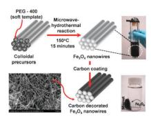
Scheme 1 Schematic illustration of the microwave-hydrothermal synthesis of single-crystalline  $Fe_3O_4$  nanowires, employing PEG-400 as a soft template and subsequent carbon decoration for application as high performance anode in lithium ion batteries.
