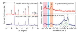
Fig. 2 (a) X-ray diffraction and (b) Raman spectra of  $Fe_3O_4$  nanowires before and after carbon decoration.
