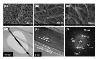
**Fig. 1** Morphological characterization of  $Fe_3O_4$  nanowires: (a) low and (b) high magnification FE-SEM images of as-synthesized  $Fe_3O_4$  nanowires, (c) FE-SEM image of carbon-decorated  $Fe_3O_4$  nanowires, (d) TEM and (e) HRTEM images showing crystalline  $Fe_3O_4$  nanowires surrounded by amorphous carbon, and (f) FFT image of single-crystalline  $Fe_3O_4$  nanowire. The subscript DD refers to double diffraction.
