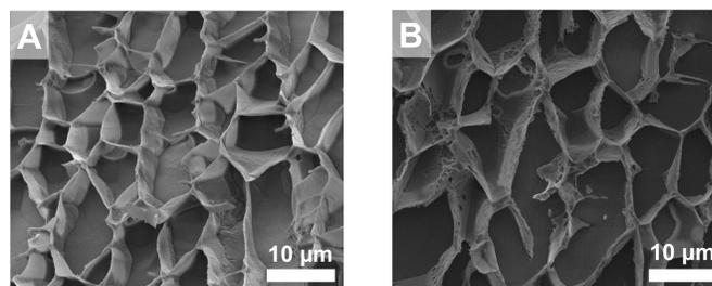
**Figure 4** (A) Cryo-SEM micrographs of the porous network formed within the 4% **PSP-POG7** and (B) 4% **PSP-POG9** hydrogels.
