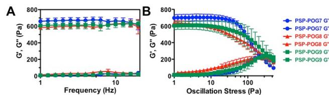
**Figure 2.** (A) Frequency and (B) oscillation stress sweep profiles comparing the 4% PSP-POG hydrogels using rheometry at room temperature.
