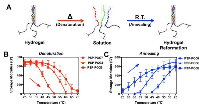
**Figure 3** (A) Schematic of the denaturation-annealing cycle of the triple helix within the hydrogel. Effect of temperature on the storage modulus of the 4% PSP-POG hydrogels (B) with increased temperature and (C) with cooling back to room temperature.
