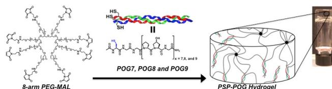
**Figure 1** Design of thermosensitive PSP-POG hydrogels based on two components: an 8-arm PEG-MAL polymer and Cys-modified collagen triple helical peptides with varying POG repeats.
