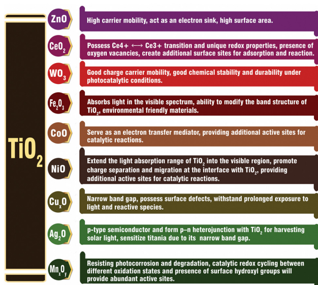
Fig. 9 Schematic representation of various metal oxides used for improving the photocatalytic hydrogen evolution activity of TiO 2 .
