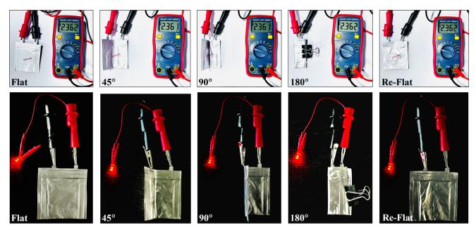
Fig. 7 Upper row: digital pictures of the OCV for the pouch cell consisting of the  $g-C_3N_4-CNT/S$  cathode at different folding angles and bottom row: pictures of LEDs lit up by the pouch cell at different folding angles demonstrating the excellent flexibility of the developed pouch cell.
