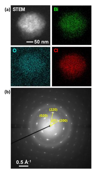
**Fig. 6** (a) STEM image and EDS mapping of a synthesized BiOCl particle, with bismuth in green, oxygen in blue, and chlorine in red. The oxygen signal is high outside of the particle due the oxygen in water. Scale bar applies for all four images. STEM image field of view is 289 nm  $\times$  289 nm (802  $\times$  802 pixels) with an EDS signal binning factor of 2. (b) SAED pattern of particle in (a) with reflections indexed.
