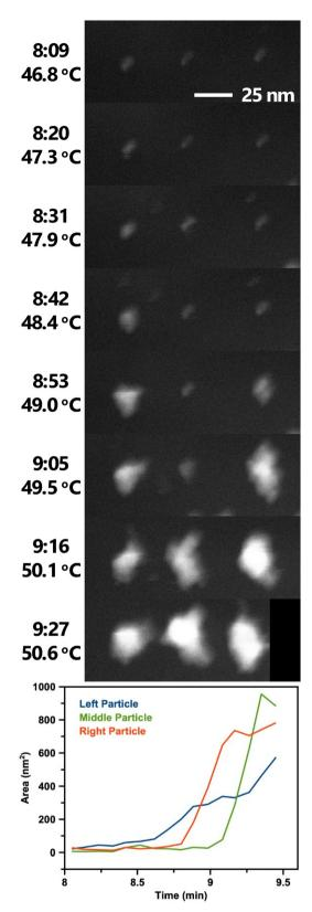
Fig. 7 Selected STEM images from Movie 2† showing BiOCl formation and growth from BiClLac. Images are spaced ca. 11 s apart with times and temperatures indicated. The black area in the last frame is where the particle clusters drifted near the edge of the field of view and was applied during drift correction. Scale bar applies to all images. Below the images is a plot of the clusters' 2D area over time. Image processing steps for Movie 2 are shown in Movie S1.†
