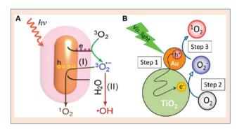
Fig. 14 Schematic representation of singlet oxygen generation from gold nanoparticles. (A) Au nanorod. Reproduced with permission.<sup>73</sup> Copyright 2014, Royal Society of Chemistry. (B) Au NP-TiO<sub>2</sub> core-shell architecture for enhanced SOG. Reproduced with permission.<sup>71</sup> Copyright 2014, American Chemical Society.
