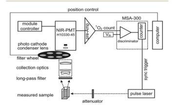
Fig. 5 Schematic diagram of the time- and wavelength-resolved  $^1\mathrm{O}_2$  luminescence detection system. $^{20}$
