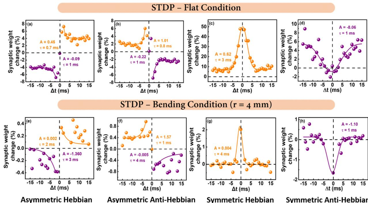
Fig. 6 Spike time-dependent plasticity (STDP) characterization of  $\text{PbI}_2$  based memristor device in flat and bending condition respectively (a) and (e) Asymmetric Hebbian, (b) and (f) Asymmetric anti-Hebbian, (c) and (g) Symmetric Hebbian (d) and (h) Symmetric anti-Hebbian.
