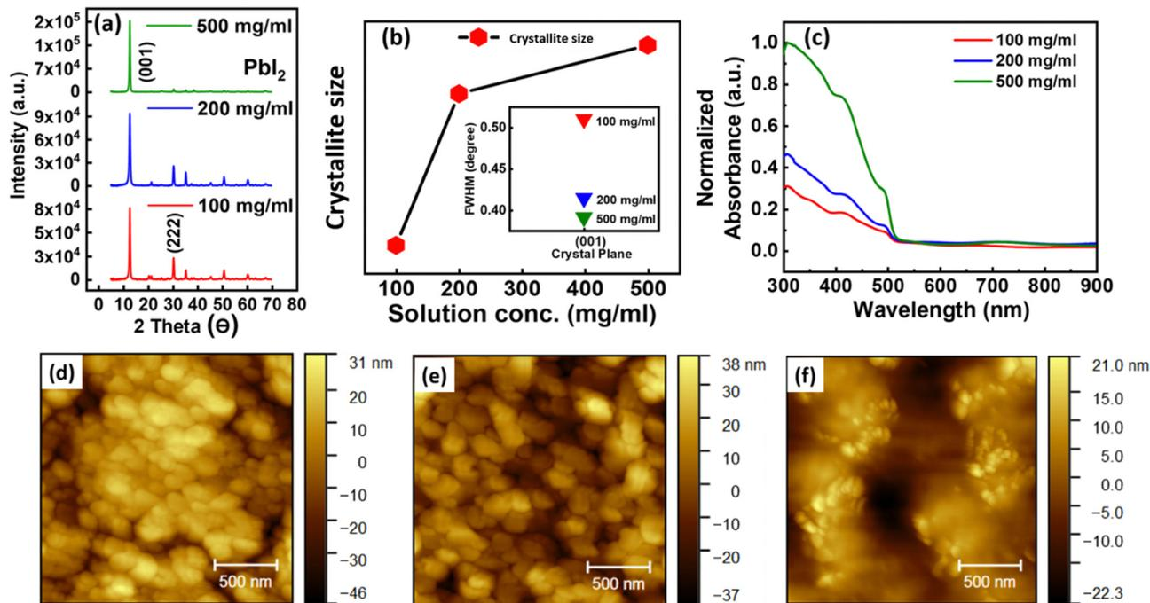
Fig. 1 (a) Series of XRD pattern of 100, 200 and 500 mg ml<sup>-1</sup> solution concentration. (b) Crystallite size extracted from XRD data, and inset represents the FWHM graph of dominant (001) crystal growth plane. (c) UV-Vis spectra of all three PbI<sub>2</sub> thin films. (d)–(f) AFM images of thin films prepared with 100, 200, and 500 mg ml<sup>-1</sup> solution concentration, respectively.
