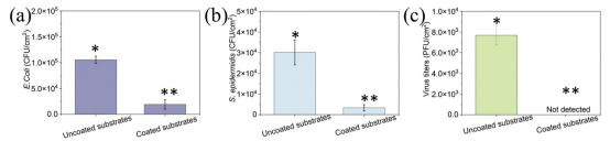
Fig. 5 The antifouling activity of uncoated and coated 3D-printed elastomer substrates against (a) E. coli and (b) S. epidermidis. The antiviral activity of uncoated and coated 3D-printed elastomer substrates against (c) bacteriophage T4. SD is based on 9 repeats. ANOVA and Duncan's test were used to indicate the statistically significant differences among values (P < 0.05).
