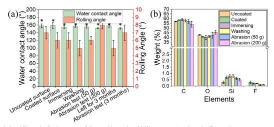
Fig. 4 Mechanical stability and adhesion assays of the peptide coating. (a) Water contact angle and rolling angle measurements after immersing, washing, and abrasion treatments, ANOVA and Duncan's test were used to indicate the statistically significant differences among values (P < 0.05), and (b) EDS analysis of 3D-printed elastomer substrate after immersing, washing, and abrasion treatments containing carbon, oxygen, silicon, and fluorine atoms.
