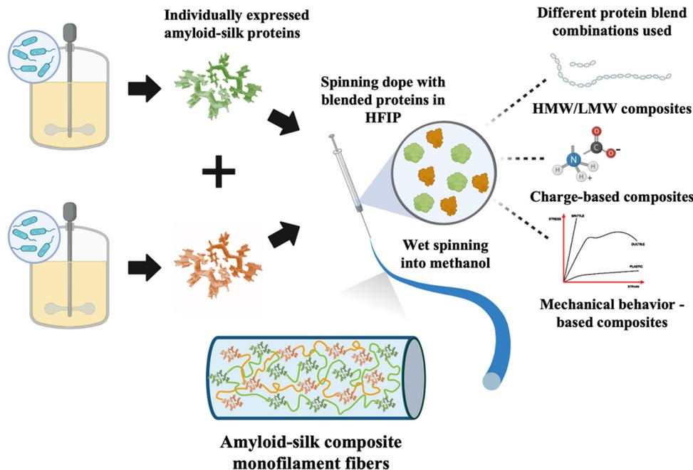
**Fig. 1** Schematics of recombinant protein-based composite fiber production. The polymeric amyloid-silk proteins were biosynthesized in engineered bacteria and purified before being blended into the spinning dope. The dopes were extruded into a coagulation bath to form monofilament composite fibers. Three different protein blend combinations were used to generate unique composite fibers – HMW/LMW composites, opposite charge composites and mechanical behavior-based composites.
