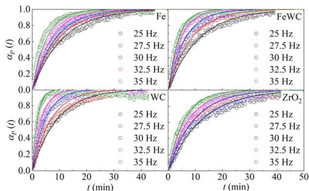
Fig. 2 The molar fraction of deuterated benzoic acid,  $\alpha_p(t)$ , as a function of time,  $t$ . Data refer to the BM experiments performed using balls made of different materials. Best-fitted curves are shown.
