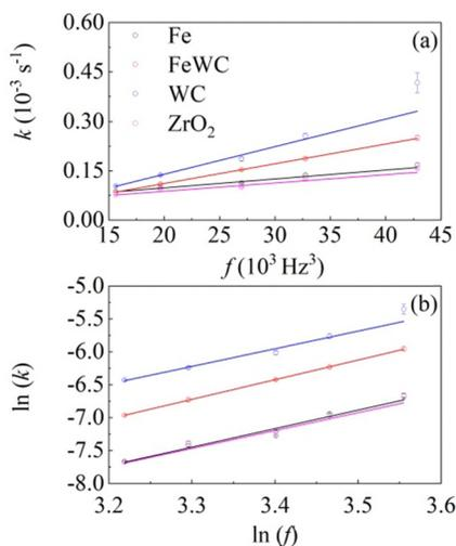
Fig. 3 (a) The volume fraction of powder that undergoes CLCs in the unit time,  $k$ , as a function of the third power of the milling frequency,  $f$ . Data refer to the BM experiments performed using balls made of different materials. Best-fitted lines are also shown. (b) The logarithmic plot of  $k$  as a function of  $f$ . Best-fitted lines have a similar slope of about 3.
