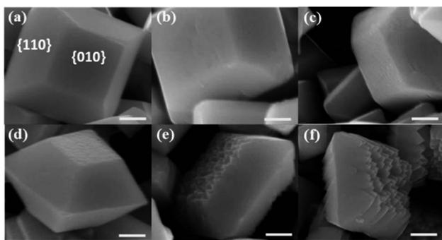
Fig. 2 SEM images of BiVO<sub>4</sub> samples etched in NaOH solution with different concentrations. (a) 0 M; (b) 0.1 M; (c) 0.2 M; (d) 1.0 M; (e) 2.0 M and (f) 3.0 M. Scale bar, 500 nm.
