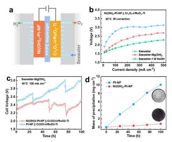
Fig. 6 (a) A schematic illustration of a direct seawater electrolyser equipped with an Ni(OH)<sub>2</sub>-Pt-NF electrode. (b) The polarization curves of an Ni(OH)<sub>2</sub>-Pt-NF-electrode-equipped electrolyser in different electrolytes. (c) Galvanostatic discharge curves of electrolysers at a current density of 100 mA cm<sup>-2</sup> and (d) mass of precipitation on the Ni(OH)<sub>2</sub>-Pt-NF and Pt-NF electrodes (inset: photographs of the HER electrodes after 100 h of measurement)
