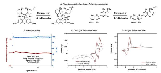
Fig. 9 (A) Electrolyte charging and discharging processes. (B) Flow cell cycling of 25 mM 4aD and 4-DMPP. (C) Cyclic voltammograms of catholyte recorded before and after cycling at 100 mV s $^{-1}$  and an initial positive scanning direction. (D) Cyclic voltammograms of anolyte recorded before and after cycling at 100 mV s $^{-1}$  and an initial negative canning direction.
