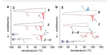
Fig. 2 DSC plots of compounds (a) 2 and (b) 5 as E and Z isomers measured during the first heating and cooling cycles. Further heating of the Z isomers results in  $Z \to E$  isomerization and heat release (exotherm highlighted in blue).
