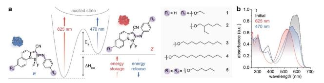
Fig. 1 (a) Chemical structures of Azo-BF<sub>2</sub> derivatives and the diagram of visible-light-triggered photon energy storage and release processes in the solid state. (b) UV-Vis spectral changes upon the photo-irradiation of compound 1 in dichloromethane (2  $\times$  10<sup>-5</sup> M).
