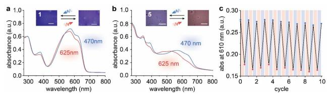
Fig. 3 UV-Vis absorption spectra and optical microscopy images of thin films (a) 1 and (b) 5 upon irradiation at 625 nm (15% 1-Z; 70% 5-Z at PSS) and at 470 nm (17% 1-Z; 48% 5-Z at PSS). Scale bar = 1 mm. (c) Isomerization cycles of thin film 5 upon alternating irradiation at 625 nm for 10 min (red filled area) and at 470 nm for 1 min (blue filled area), monitored by the absorbance changes at 610 nm.
