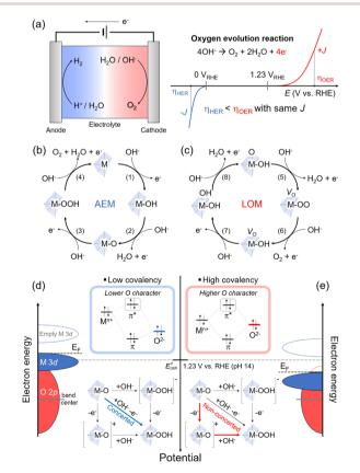
Fig. 2 Two principal OER processes. (a) Schematic illustration of the water splitting cell and I-V curve for the HER and OER. Mechanism scheme of the 4-electron transferring oxygen evolution reaction by (b) the adsorbate evolution mechanism (AEM) and (c) lattice oxygen mediated (LOM) pathway. Schematic band diagram of (d) low covalent and (e) high covalent transition metal oxides. The concerted and nonconcerted one-electron transfer processes are illustrated, respectively.
