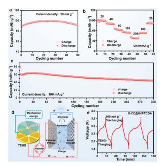
Fig. 5 Electrochemical performance of PTCDA//O-CC@K full cells. (a) Cyclic performance at 20 mA g $^{-1}$  and (c) rate performance at different current densities; (c) long-term cyclic performance at 100 mA g $^{-1}$ ; (d) schematic of TENG charge and galvanostatic discharge of the self-powered system; (e) TENG charge and galvanostatic discharge performance of the self-powered system by O-CC@K//PTCDA batteries. All cells were tested after a 20-cycle activation process at 20 mA g $^{-1}$ .
