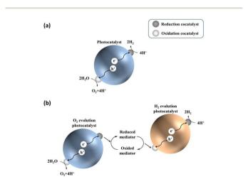
Fig. 1 Schematics of (a) one-step-excitation and (b) two-step-excitation (Z-scheme) overall water-splitting processes.
