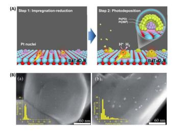
Fig. 4 (A) Schematic of sequential Pt cocatalyst deposition onto  $BaTaO_2N$ . Adapted with permission from ref. 40. Copyright 2021 Springer Nature. (B) Scanning transmission electron microscopy images and particle size distributions of (a) Na-containing and (b) Nafree Pt/BaTaO\_2N. Adapted with permission from ref. 41. Copyright 2021 The Royal Society of Chemistry.
