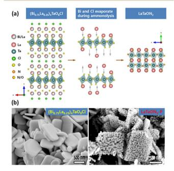
Fig. 2 (a) Schematic of structural transformation from  $(Bi_{0.75}La_{0.25})_4$ - $TaO_8Cl$  into  $LaTaO_2N$ . (b) Field-emission scanning electron microscopy images of  $(Bi_{0.75}La_{0.25})_4$ TaO $_8Cl$  and  $LaTaON_2$ -P. Adapted with permission from ref. 21. Copyright 2021 American Chemical Society.
