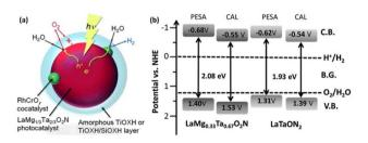
Fig. 6 (a) Schematic of the OWS reaction mechanism on surface-coated RhCrO $_x$ /LaMg $_{1/3}$ Ta $_{2/3}$ O $_2$ N. Adapted with permission from ref. 46. Copyright 2015 Wiley-VCH. (b) Band levels for LaMg $_x$ Nb $_{1-x}$ O $_{1+3x}$ -N $_{2-3x}$  (x=0 and 0.33) estimated by theoretical calculations (CAL) and photoelectron spectroscopy in air (PESA). Adapted with permission from ref. 47. Copyright 2016 The Royal Society of Chemistry.
