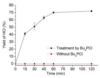
Fig. 4 Yield of HCl, determined by acid-base titration, during reaction of PVC with 0.85 eq.  $Bu_4PCl$ , 2 mol% Rh at 180 °C in butanone, with rapid dehydrochlorination during the initial 60 minutes. Error bars represent the standard deviation. Control reaction of PVC without  $Bu_4PCl$  in butanone yielded no HCl (conditions: 1 mmol PVC, 180 °C, 20 bar  $H_2$ , with 2 mol% H(CO)Rh(PPh<sub>3</sub>)<sub>3</sub>).
