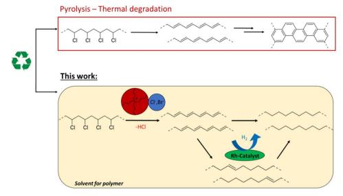
Fig. 1 Recycling of PVC. (top) Polyacetylenes, formed *via* pyrolysis and thermal degradation tend to crosslink to polyaromatic tar. (bottom) Solvent based tandem dehydrochlorination—hydrogenation, using ionic liquids and Rh catalysts, can lead to saturated polymers.
