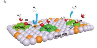
Fig. 1 (A) The reaction mechanism for the HER in alkaline electrolytes and two pathways are presented in the forms of the Volmer–Heyrovsky mechanism and the Volmer–Tafel mechanism. (B) Schematic diagram of synergetic catalysis of alloy–oxide or alloy–hydroxide interface structures, in which the oxide or hydroxide promotes water dissociation and the alloy accelerates hydrogen combination.
