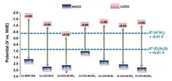
Fig. 3 Energy level diagram vs. NHE and vacuum of substituted Ce-UiO-66-X and MOF-808(Ce) materials as well as Zr-UiO-66-NH<sub>2</sub> and Zr-UiO-66-NO<sub>2</sub> taken as reference compounds.<sup>41</sup> The figure also indicates the required potential for the HER or OER vs. NHE at pH 7.
