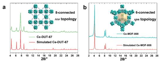
Fig. 2 PXRD patterns ( $\lambda_{Cu} = 1.5406$  Å) of synthesized (a) 8-connected *reo* Ce-DUT-67(PDA) and (b) 6-connected *spn* Ce-MOF-808 in comparison to simulated patterns, insert images: structure schemes of the corresponding MOFs.
