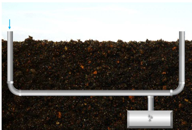
Fig. 13 Schematic of condensation drinking water production method.
